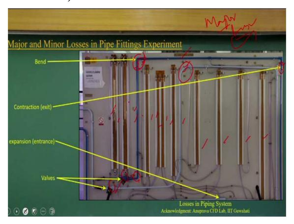
On the next slides what I am showing it that how we conduct the experiments to quantify the how much of losses are happening, energy losses is happening it. So one if you look it, we call major losses. Major losses, that is the losses due to the frictions. So that way if you look it there are the two pipes are there. And in these two different pipes there are the manometers are attached to determine what is the pressure difference at the two points, you just closely look it.
