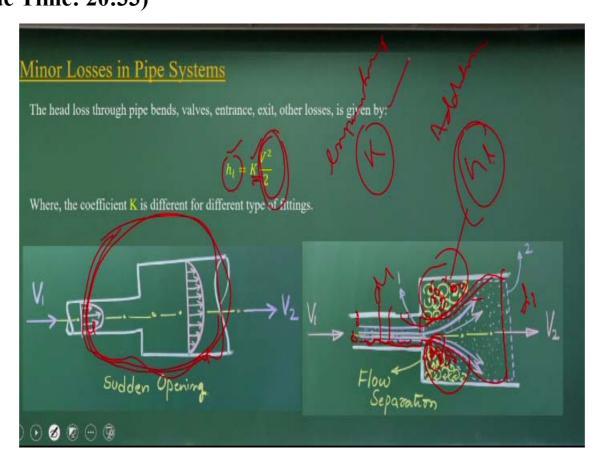
Now let us go to the minor losses in the pipe systems. As I told it when you have the pipes, it can have a regions you have a smaller pipe to bigger pipe or bigger pipe to the smaller pipe. When you have a these conditions that means the flow is coming it here and going out, the smaller diameters and the larger diameter. If you have these conditions, what we do it that when you compute the energy losses, for this total regions, we compute the analysis this.
